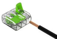
Termination: Lift the lever to open the clamping unit and insert a stripped conductor
