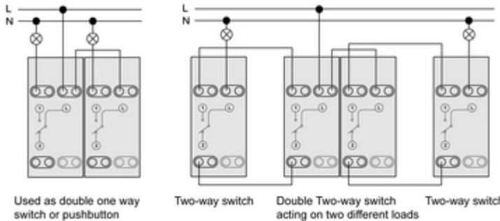
Used as double one way switch or pushbutton
