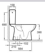
Descriptif CCTP: Pack cuvette SANS BRIDE sortie verticale. E22919. Collection: PATIO. DIMENSIONS: 78,70 x 38,50 cm. POIDS: 38,8 kg. MATÉRIAU: Céramique. TYPE D'INSTALLATION: Au sol. CONSOM-MATION D'EAU: Standard 3/6 L. HAUTEUR: Standard. TYPE DE BRIDE: Sans bride.
